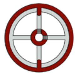
Bored Hole With 2 Setscrew Holes at 90°
