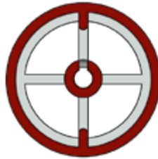
Bored Hole With Setscrew Hole Over Keyway
